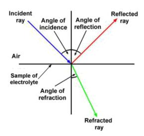
Total internal reflection is the return of the light waves (incident rays) after they have struck the surface of the electrolyte sandwiched between the measuring prism and cover plate.
