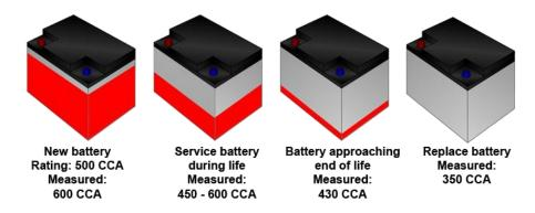
These conditions significantly degrade the performance of the battery and can be measured through its conductance value.
