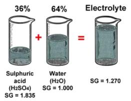
A fully charged battery has a high Sulphuric acid (H<sub>2</sub>SO<sub>4</sub>) concentration in the electrolyte and therefore a high specific gravity because the chemical reaction used to produce an electrical charge has not broken down the acid.
